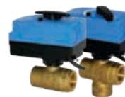
Conski ventili (2- / 3-potni) s pogoni serije 9000: -z zunanjim navojem (holandci) (G3/4" - G1 1/2") -z notranjim navojem (Rp 1/2" - Rp 1 1/4") -compression fitting (CPF22mm, CPF28mm)
